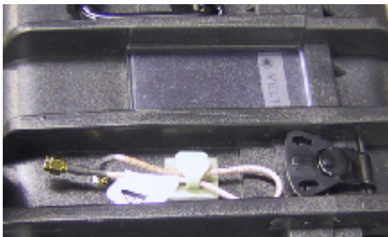
External, wireless antenna connection
