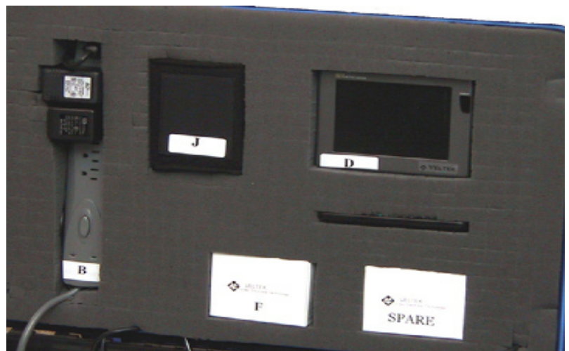
Inside lid houses (from left to right) a power strip, optional serviceman's monitor, Model VCT64LCD (6.4" LCD monitor). 2 optional color board camera kits are shown below the monitor.
